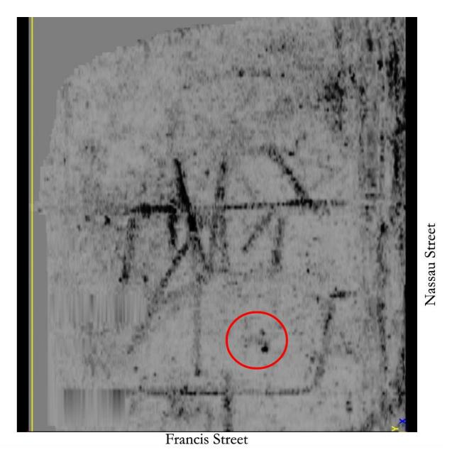
Figure 10: GPR timeslice of the southern survey area. The large linear anomalies represent early  $20^{th}$  C. drains, the red circle marks the location of the "H" shaped chimney base.
