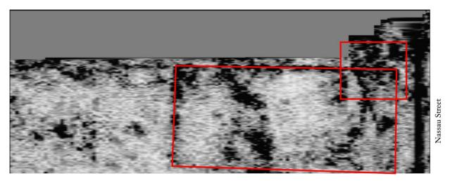
Figure 9: GPR timeslice of northern surveyed area. The large red box represents a line of anomalies likely associated with the foundations of the 1855 brick church structure, the smaller red box represents anomalies potentially associated with the earlier brick foundations identified during the 1957 excavation.
